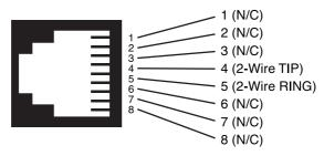
Figure 5. Model 1082 RJ-45 twisted pair line interface
